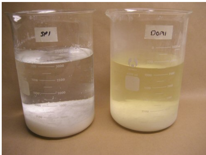
12. A batch of Spanish and a batch of Domestic, cooled to 0C just prior to the second filtering
