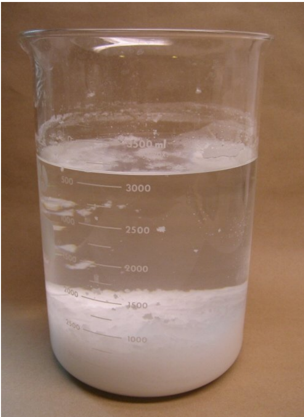
2 A beaker of HP-140 that has been filtered and cooled showing the precipitated \text{KClO}_4 crystals
